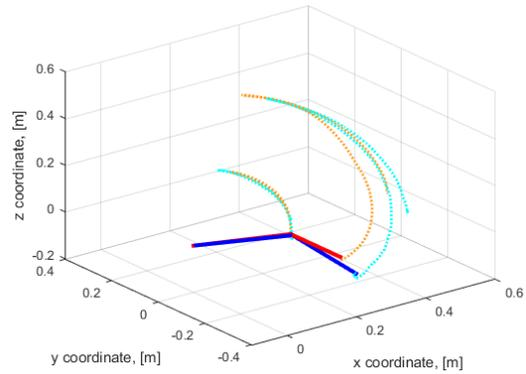
Fig. 9. Arm trajectory comparison: blue/cyan lines represent 4-DOF arm tracker, red/orange - Xsens MVN suit. Solid lines represent arm segments, dotted lines - trajectories.
