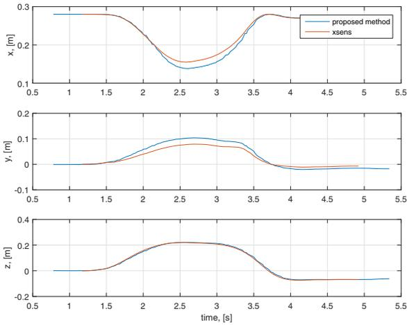
Fig. 7. Elbow coordinates generated by 4-DOF arm tracker and Xsens MVN suit during a motion
