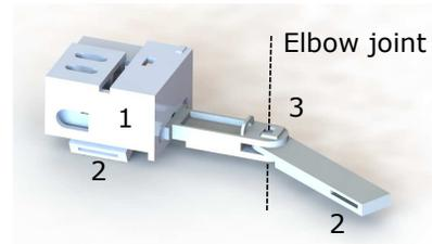
Fig. 2. CAD model of 4-DOF wireless arm tracker: 1 - IMU case, 2 - Velcro strip holes, 3 - two-link potentiometer holder
