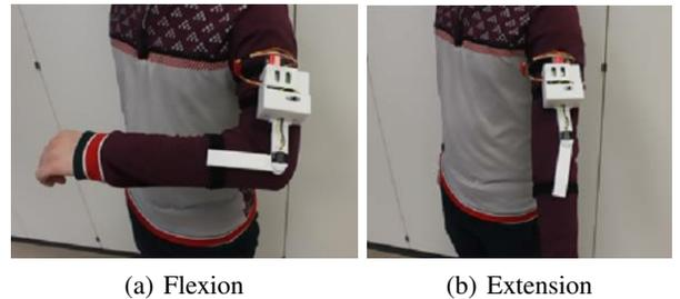
Fig. 3. 4-DOF wireless arm tracker mounted on a user with different arm poses
