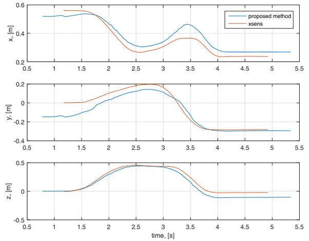
Fig. 8. Wrist coordinates generated by 4-DOF arm tracker and Xsens MVN suit during a motion
