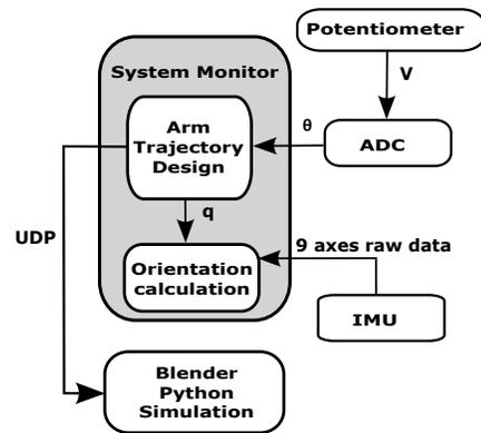
Fig. 6. PC based control system of 4-DOF Wireless arm tracker
