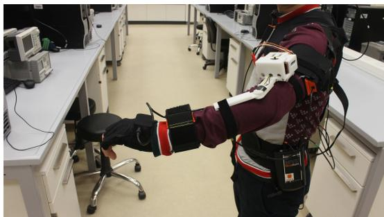
Fig. 5. 4-DOF arm tracker system prototype and Xsens MVN suit on a human user for comparative analysis
