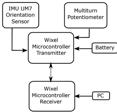
Fig. 4. Communication loop of 4-DOF wireless arm tracker
