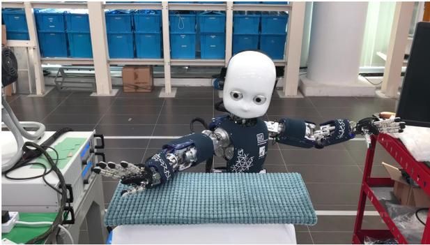
Fig. 4: Experiment setup using the iCub robot. The material is fixed on a non-deformable metal surface and taxels on the iCub forearm are used to collect the tactile data.
