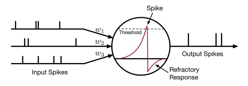
We use **Spike Response Model (SRM)** as a neural model. Spikes are generated when membrane potential u(t) exceeds a predefined threshold  $\phi$ . The neuron in **SRM** depends on the incoming spikes to be convolved by a response kernel,  $\epsilon(\cdot)$ , and refractory response,  $v(\cdot)$ :
