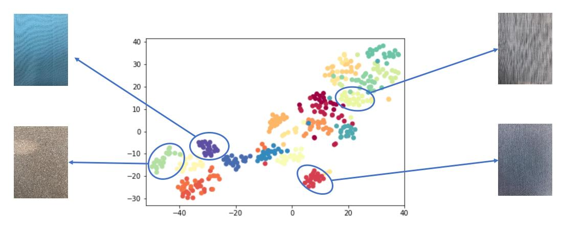
t-SNE performed on encoded iCub tactile data using Van-Rossum distance. The clusters are visually separable. Some examples of clusters are indicated with respective textures.
